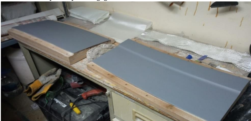
Figure 1. Schematic of joint mould to manufacturing a sandwich panel joint
