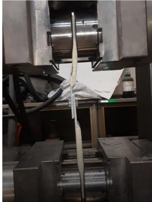
Figure 3. Experimental process of edge-wised compression test and failure modes
