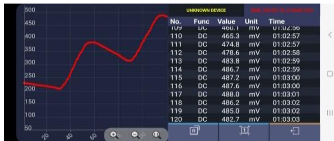
Figure 1. The output voltage of a sample thermoelectric module recorded by the data logger.
