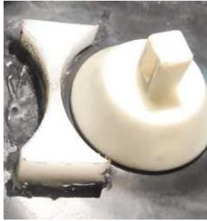
Figure 3. Final optimized obstacle design installed on the diaphragm.
