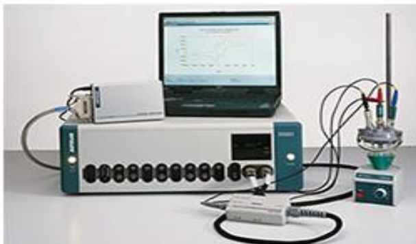
Figure 4. Conventional electrochemical cell arrangement in the three-electrode system.
