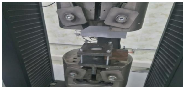
Figure 2. Built-in fittings sample test fixture and Galdabini tensile testing machine.
