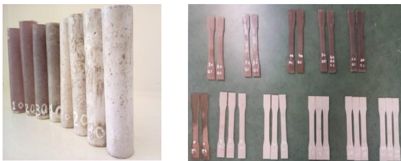
Figure 1. The samples prepared for measuring the thermal conductivity and mechanical properties under tensile loading.
