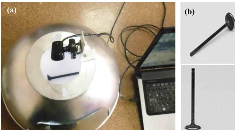
Figure 1. (a) Lighting chamber with a camera; (b) a sample of the valve under test.
