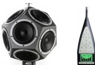
Figure 1. Right: 2260 B&K Sound level meter; Left: omni directional speaker.
