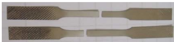
Figure 1. Tensile test samples after the test.
