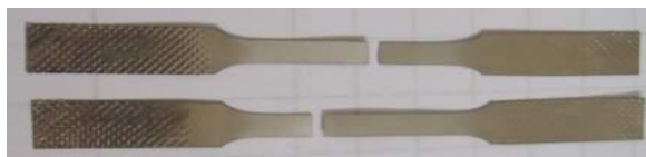
Figure 1. Tensile test samples after the test.
